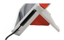
**#2:** Connect the magnetic power supply to the ExpressPoll and plug the power block into an outlet.
