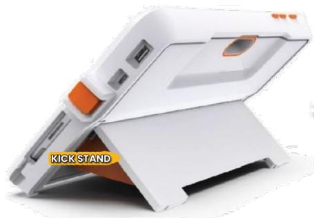
1. To prepare the flip stand for use, first **open the kick stand** to reveal two orange brackets. Lift each bracket to free them from their white clasps.
