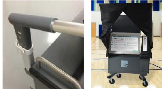
5. **Adjusting Touch Screen Angle.** Initially adjust screen angle after transport by holding the top and bottom of the screen and tilting to an angle that is comfortable for most voters. To ensure proper function, voters should adjust the screen to their preferred angle in the same manner. The screen should be adjusted to the vertical position for voters in wheelchairs.
