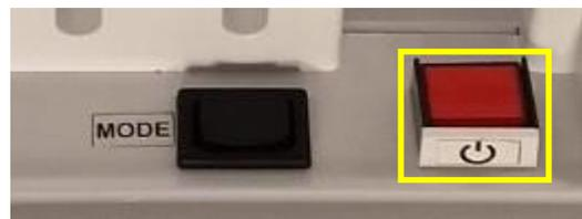
Unlock and open the Access Compartment door on top of the terminal. Inside the Access Compartment, press and release the red power button. Once the red power button is pressed, a yellow alert will appear on the screen letting the operator know the machine is not ready for voting because the media door is
